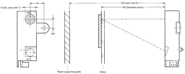
Note: 1. The part with oblique lines indicates the paper sensing area of the EY3A-1081, which is practically determined by the diameter of the beam and its tolerance.
