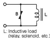
2. The cable for connecting the surge suppressor must be as short as possible in length, and thick enough in diameter so that it can sufficiently withstand the surge current. The short length and thick diameter are important to reduce the inductance and generated voltage, and to protect the device from heat damage.
