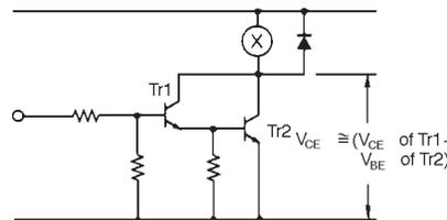
When the Darlington-connected transistors are used, the required value of  $V_{CE}$  is higher than when using a single transistor. For this reason, consideration must be given to designing the total power dissipation and supply voltage for the second transistor, Tr2.
