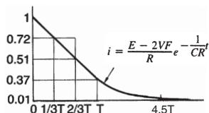
Voltage drop E1 across the total resistance of the capacitance C's resistance and relay coil's internal resistance is the difference between the supply voltage E and voltage drops across two diodes: Di1 and Di2. Hence,
