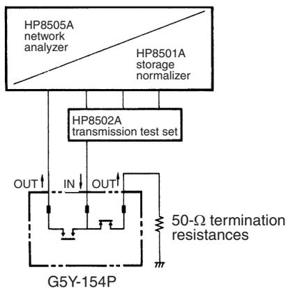
The following characteristics are measured with contacts unrelated to the measurement terminated at 50Ω, when a signal is applied from input terminal 11 to output terminal 8 or from input terminal 11 to output terminal 14 of the sample.
