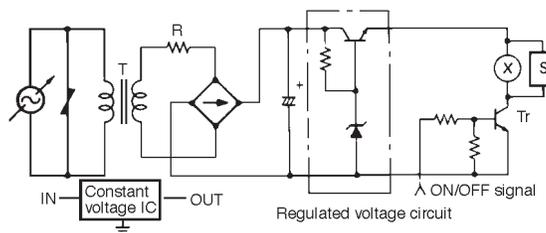
Relays consume more power than semiconductor elements. The following circuit configuration is recommended to improve the characteristics.
