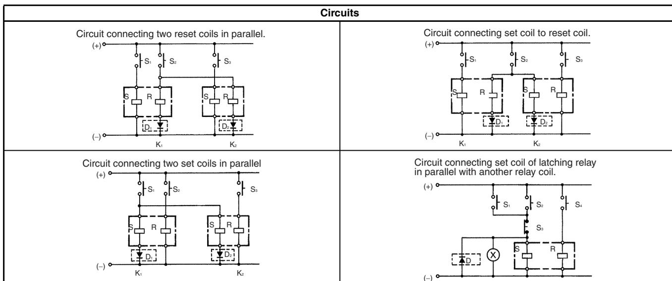
When connecting a diode to the relay circuit, be sure to use a diode with a repetitive peak-inverse voltage, and a DC reverse voltage sufficient to withstand external noise or surge. Also be sure that the diode has an average rectified current greater than the coil current.
