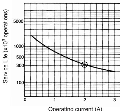
However, with a DC load, it may become difficult to break the circuit of 48 V or more due to arcing. Determine the suitability of the relay in actual usage testing.
