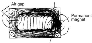
When the switching voltage is removed from the coil, the collapse of the magnetic flux created by the permanent magnet and the electrical coil provides the force to return the relay contacts to the reset position. Note the flux path and magnet polarity in the illustration overleaf.
