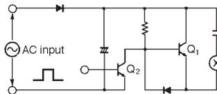
Half-wave rectified AC power is applied to the circuit. Q<sub>1</sub> is the output of a TTL, and drives the relay.
